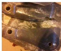
Left: the tail bump stops, top is the Port one showing the touch down wear. Right: is the Air Brake showing the damage from the runway scrape
