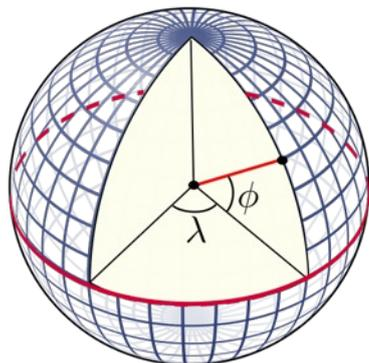
piece of which suspended from a cord acted as an early compass. Awareness of the sun's regularity led to the development of sextants to determine latitude ( $\phi$ ) vertical distance from the equator – but to fix one's location a horizontal distance, longitude ( $\lambda$ ) from a known point is required, which can be obtained by using an accurate clock and the time difference between
