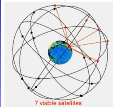
and sophisticated equipment is used to work out errors created by natural phenomena. There are 3 main systems in use: Navstar (USA), Glonass (Russia) and Galileo (Europe) about 30 satellites each, in multiple orbits, to ensure that enough satellites are 'visible' to obtain bearings.
