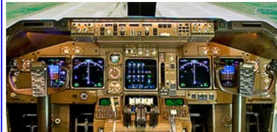
Electronic Flight Information System. Each panel could show multiple items of information and the central panels could be switched to
