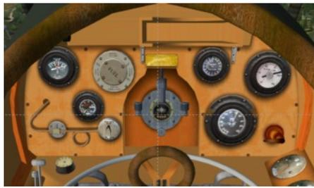
with perhaps half a dozen gauges covering the basics of height, turn and slip, speed, fuel quantity, rev counter, oil pressure with a few valves and levers to complete. This was
